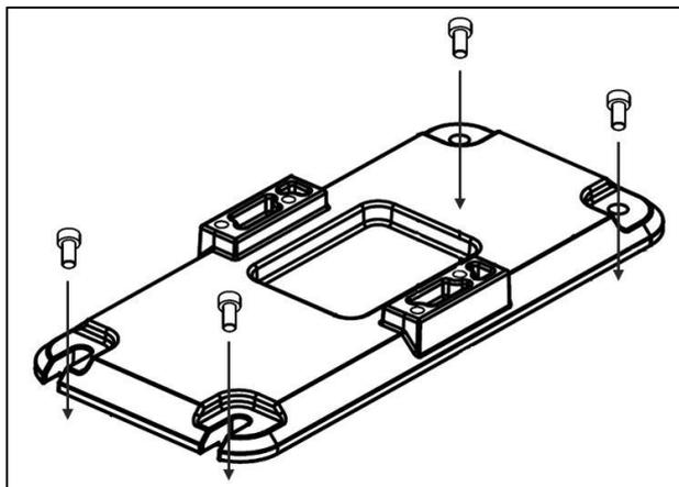
Fig. 7 Pump mounting
