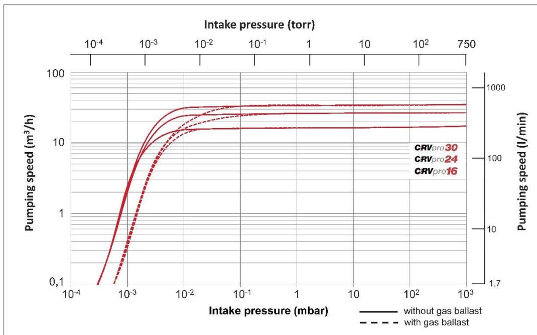
Fig. 5 Pumping Speed / Intake Pressure - Diagram CRVpro 16, 24, 30
