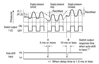
When the auto-shift function is selected, " $\Re S_{10} = 0.00$ " will be displayed on the sub screen for about 1 second, and the pressure value at that point will be saved as reference value " $\mathcal{E}_{-}S$ " Based on the saved reference value, output on-off points controlled by set values\*2 such as " $\mathcal{P}_{-}I_{1}$ " " $\mathcal{H}_{-}I_{1}$ " " $\mathcal{P}_{-}Z$ " and " $\mathcal{H}_{-}Z$ " will also be rectified.
