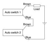
When two auto switches are connected in series, a load may malfunction because the load voltage will decline when in the ON state.
