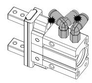
When elbow piping fittings are used, they may interfere with each other or part of gripper, limiting the range for piping entry. Please use extended male elbow, KQ2W, or extension fittings listed in the table below to avoid this situation.
