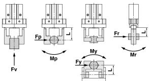
L: Distance to the point at which the load is applied [mm]
