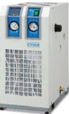
IDH thermal air dryer It reliably removes condensation from the compressed air and controls the temperature it at the same time
