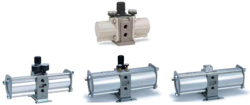
VBA booster regulator It boosts the pressure of compressed air by four times, power-free operation
