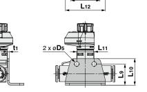
**DIN Rail Mounting Bracket** Bracket on a single side AS1002FSM/FSC AS2002FSM/FSC  $2 \times \alpha \mathbf{D} \mathbf{f}$ L18 L24 AS2052FSM/FSC
