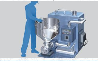
For the removal of water droplets after shower testing
