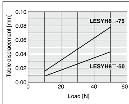
Table displacement due to roll moment load
