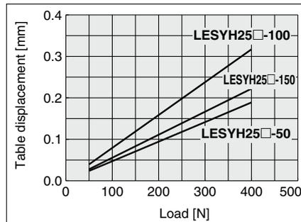
Table displacement due to roll moment load
