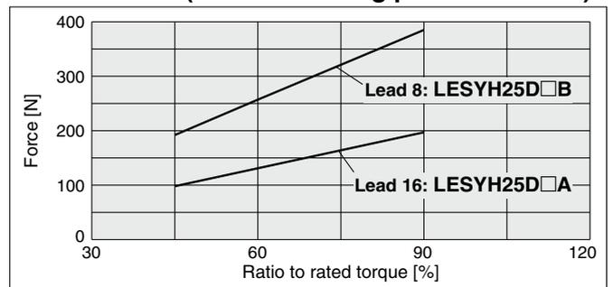
\* When using the force control or speed control, set the max. value to be no more than 90% of the rated torque.
