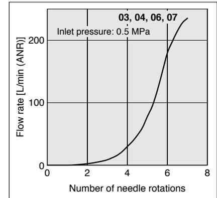
\* The numbers above the flow rate characteristic curves in the charts show the applicable tubing outside diameter as defined by the product number.
