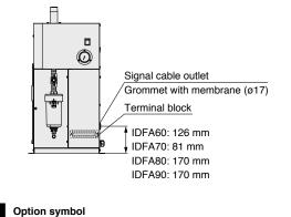
Drainage is discharged by controlling a solenoid valve with a timer. A strainer for solenoid valve protection and a stop valve are also included.
