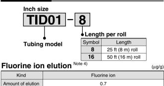
Cut the fluoropolymer tube into 15 g and clean it with pure water. After letting the 15 m/ of 25% methyl alcohol elute for 24 hours at the room temperature, dilute the elute with ultrapure water. In accordance with the dissolution method, carry out the quantitative study of fluorine ions.
