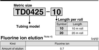
Cut the fluoropolymer tube into 15 g and clean it with pure water. After letting the 15 ml of 25% methyl alcohol elute for 24 hours at the room temperature, dilute the elute with ultrapure water. In accordance with the dissolution method, carry out the quantitative study of fluorine ions.
