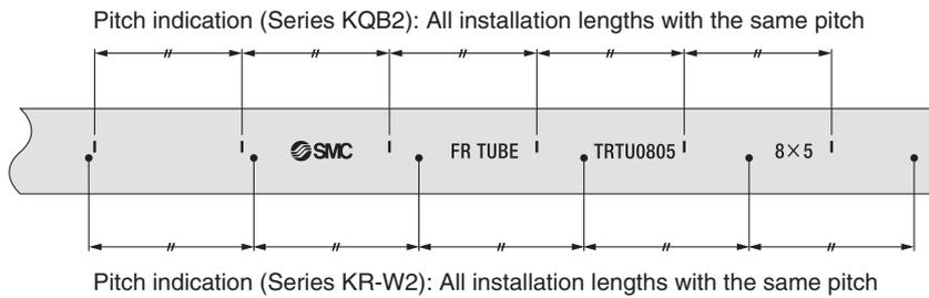
**Identification of the pitch length for installation**
