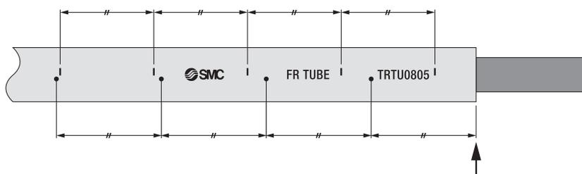
Strip off the aluminum laminated film to prevent the inner tube from being damaged.
