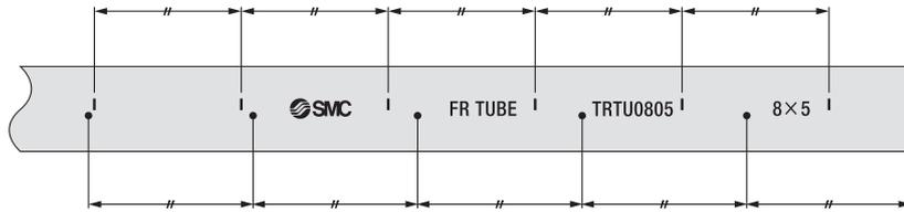
Outer layer, aluminum laminated film and inner tube are cut at the “•” mark.
