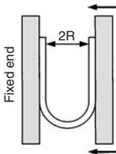
Bend the tube into the U-form at a temperature of 20°C. Fix one end and close loop gradually. Measure 2R when the deformed ratio of the tube diameter at bending reaches 5%.
