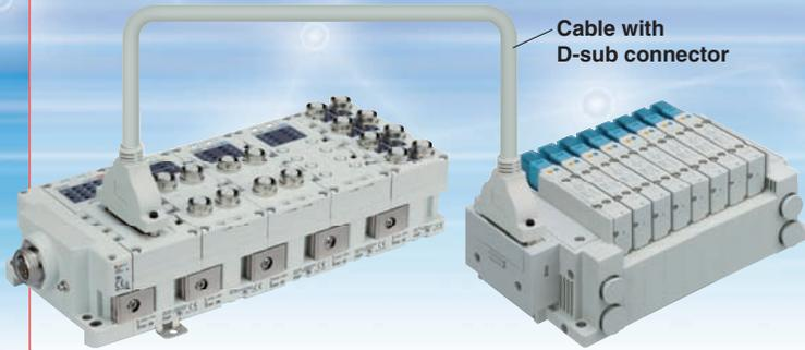
These units are capable of connection using a D-sub connector. There are three types of units, for digital input, output, and input/output. The Digital Output Unit can be connected with an SMC manifold solenoid valve F kit (D-sub connector).
