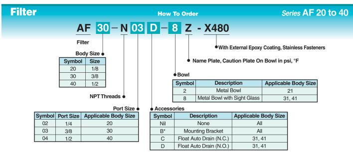
\*Note: Bracket is not assembled and is supplied loose at time of shipment.
