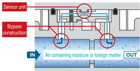
\* There is no bypass construction for the 1 and 2 L ranges.
