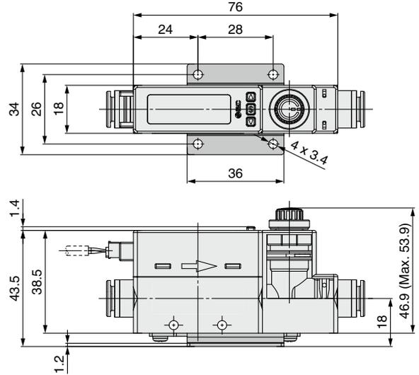
Panel mount adapter/With flow adjustment valve
