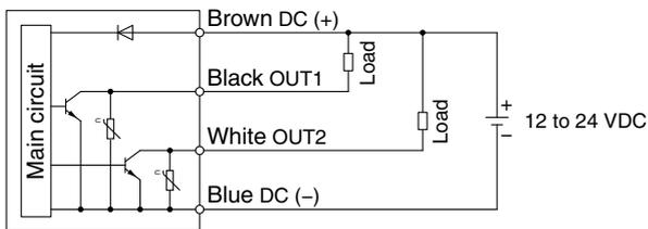
Max. applied voltage: 28 V, Max. load current: 80 mA,
