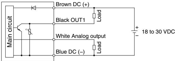
Max. applied voltage: 30 V, Max. load current: 80 mA,
