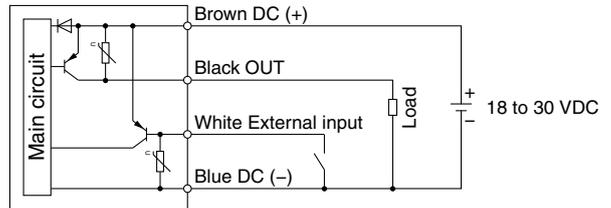
Max. load current: 80 mA, Internal voltage drop: 1.5 V or less
