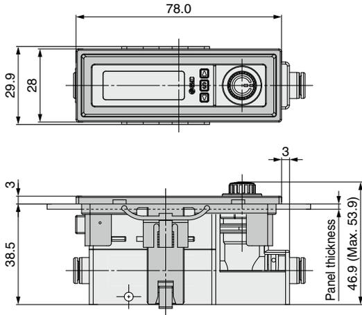
With bracket/With flow adjustment valve
