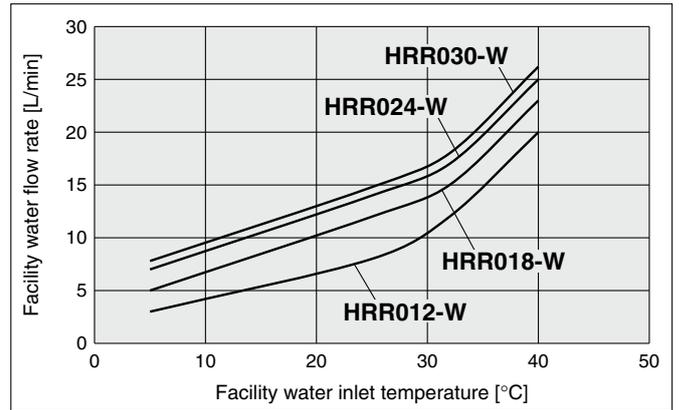
\* This is the required facility water flow rate at the circulating fluid rated flow and the cooling capacity listed in the "Cooling Capacity" specifications.
