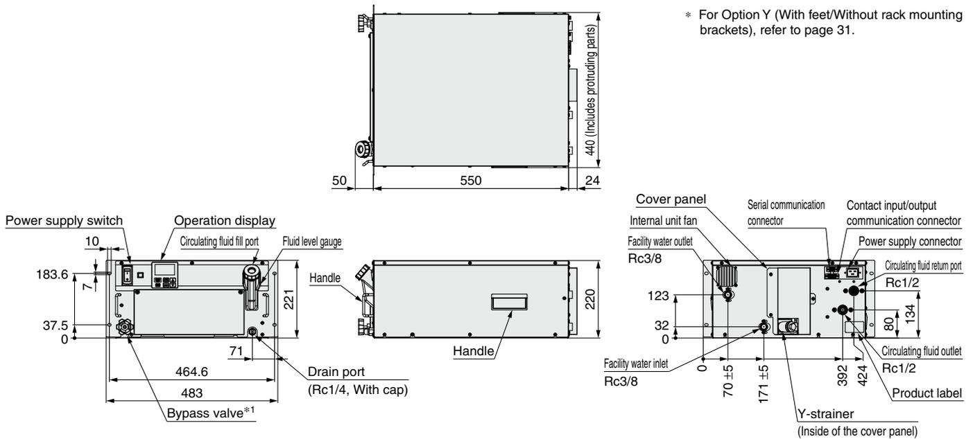
\*1 Without bypass valve for Option Z (Removed parts)
