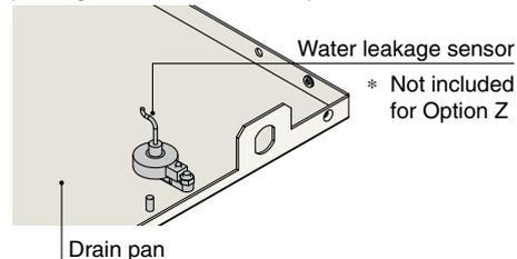
Water leakage sensor
