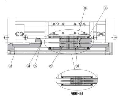
\* The numbers are the same as the "Construction" of the Best Pneumatics No.3 Series REBH.
