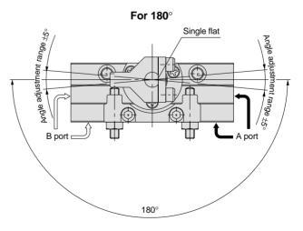
Note) • The drawings show the rotation range for the shaft's single flat.
