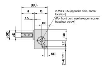
Note 2) For the  $180^\circ$  specification, the slated line area do not exist. Note 3) The maximum dimensions that appear are those measured at the maximum rotation angle settings:  $100^\circ$  and  $190^\circ.$
