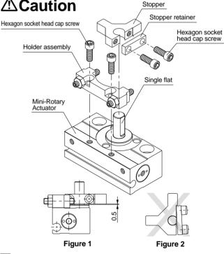
Assemble the stopper retainer to the stopper temporarily. Then place the stopper retainer in the single flat position and tighten with hexagon socket head cap screws.
