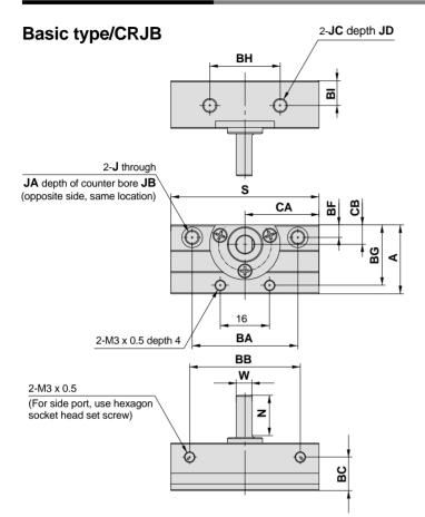
Note 1) This dimension is for the actuator with D-F9 type auto switch (not including the 2-color indication type).
