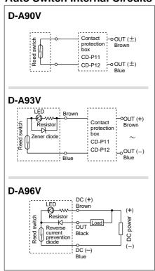
Note) 1 The operating load is inductive load.
