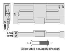
2. The plug position of the piping port can be changed to suit the operating conditions.
