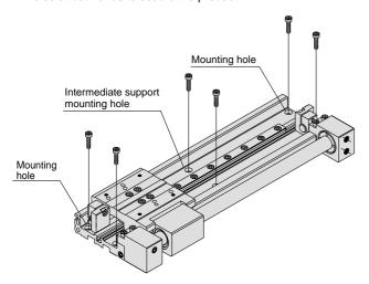
4. When a 25 mm adjustment bolt is selected, the mounting holes will be hidden behind it. Adjust the adjustment bolt after the cylinder is installed.
