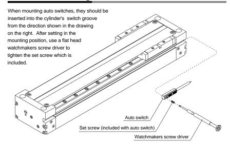
Note) When tightening the auto switch set screw (included with the auto switch), use a watchmakers screw driver with a handle about 5 to 6mm in diameter. The tightening torque should be approximately 0.05 to 0.1N·m. (0.04 to 0.07 ft • lb)
