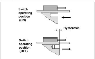
The difference between the switch operating position (ON) and the return position (OFF) is usually 2mm or less for reed switches and 1mm or less for solid state switches. However, this varies with the operating environment and is not guaranteed. Consult SMC regarding applications in which hysteresis become a problem.
