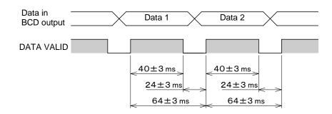
When readout enable signal is High (when output transistor is OFF), data will be valid. BCD output is continuously transmitted in the timing as shown above.
