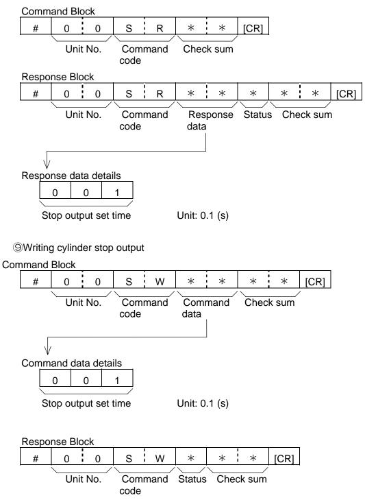
Note: Setting time for cylinder stop output is 1 (0.1 second) or more. For zero (0), error occurs.
