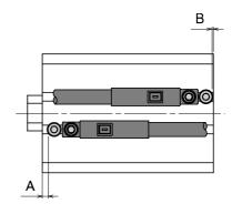
•Proper Auto switch mounting position/height (mm)
