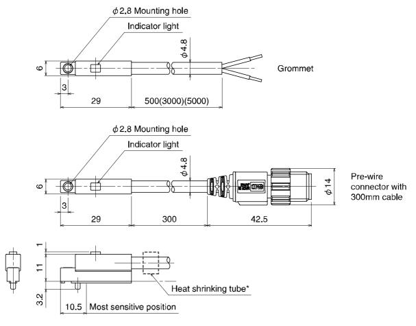
\*: Mounting the white heat shrinking tube with only D-P3DWSE.
