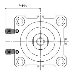
•Proper Auto switch mounting position/height
