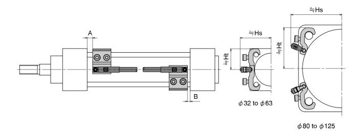
•Proper Auto switch mounting position/height
