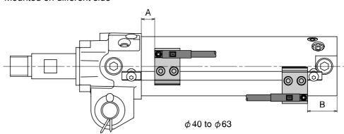
•Proper Auto switch mounting position/height
