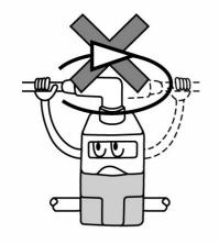
Please note that the right angled cable connector does not rotate and is limited to only one entry direction.
