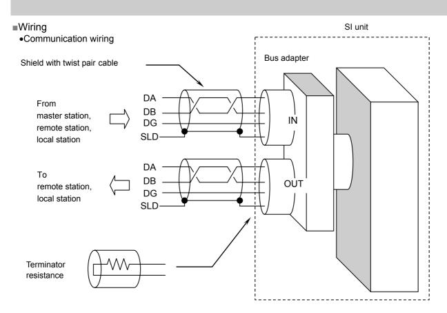
Connect the terminal resistance to the end of connection on the network. Select correct type of terminating resistance which depends on the cable type.
