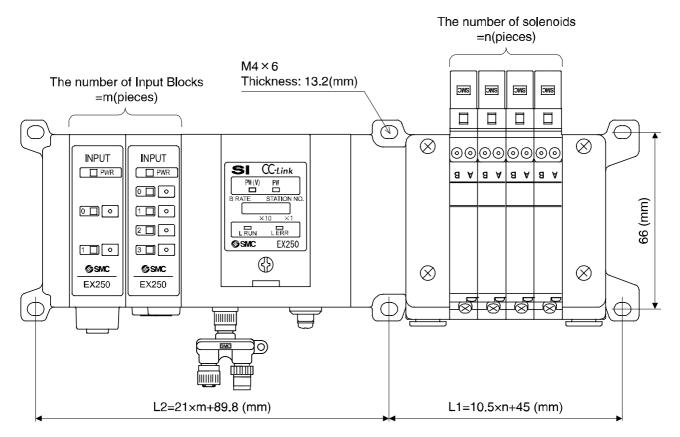
For example, the table below shows the size when manifold of VQC1000 series connected. Please refer to an individual catalog for the size when other manifolds are connected.
