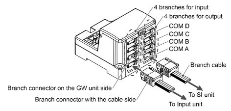
Connect the branch connectors for GW unit in order from the bottom one (COM A, B, C, and D).
