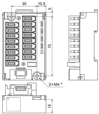
Cover removed (tolerance ±0.2 mm)
