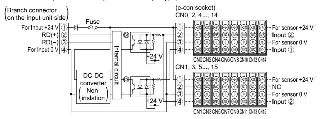
Example of wiring: D-M9N (3-wire type auto switch NPN output)
