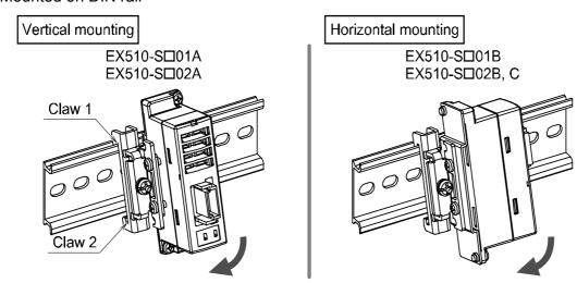
1, Hook claw 1 over the upper side and claw 2 over the low side of DIN rail respectively.
