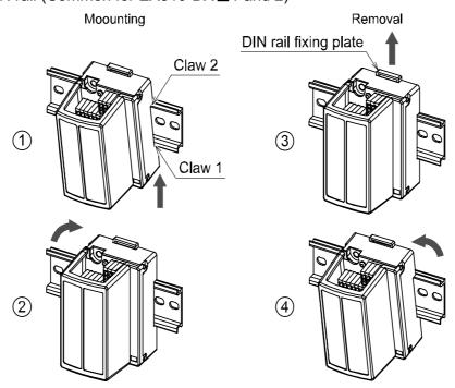
Put claw 1 at the body under DIN rail and push it upward. Push down claw 2 to the opposite rail unit the claw clicks to be set stably. (Mounting procedure ① and ②)
