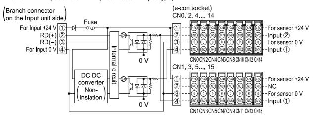
Example of wiring: D-M9P (3-wire type auto switch PNP output)
