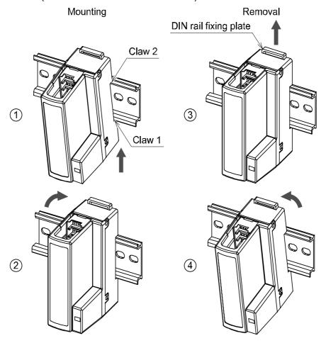
Put claw 1 at the body under DIN rail or bracket and push it upward. Push down claw 2 to the opposite rail until the claw clicks to be set stably. (Mounting procedure ① and ②)
