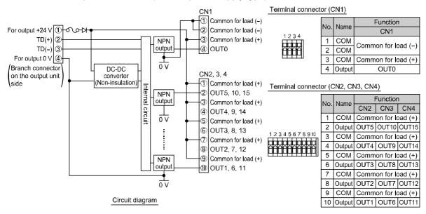
•EX510-DYN4: Output unit for NPN (Auxiliary power supply type)
