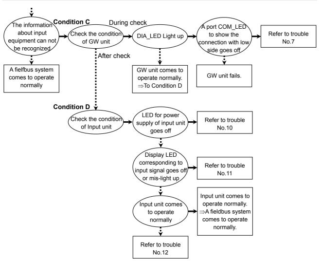
\*: Some types of output equipment do not have LED display. For such equipment, check the Output unit voltage to judge if it is normal or not.
