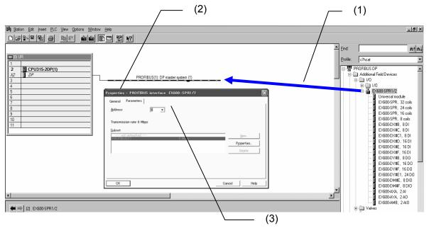
(4)Press the [OK] button to confirm the address setting. Icon of [EX600-SPR1/2] will be shown on [station] window.
