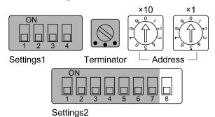
Address setting switch (x10): Sets the 10 digit of the PROFIBUS DP node address. Address setting switch (x1): Sets the 1 digit of the PROFIBUS DP node address. Settings 2 switch (8): Sets the  $3^{rd}$  digit of the PROFIBUS DP node address.
