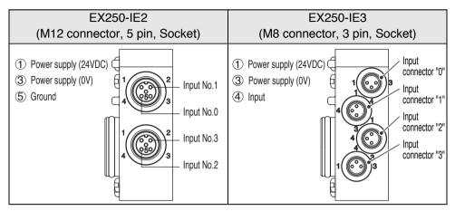
• Be sure to check the specifications of the input signal when wiring the sensor. It may cause the malfunction. Mind the position of the mounting key when selecting the sensor.
