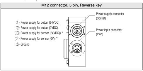
\* It is used when power is supplied to SI Unit, using an exclusive cable from the power supply connector.
