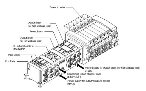
This system realizes reduced wiring between the input and output equipment by connecting to EtherNet/IP. EtherNet/IP and the input and output equipment communicates through the SI Unit.
