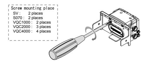
(5) Connect the SI unit and the manifold solenoid valve.
