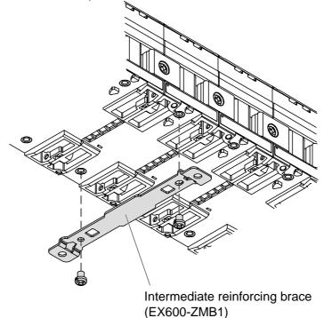
Fix and tighten the end plates at one end of the unit as shown in the figure below.
