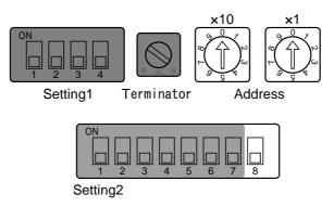
Address Setting switch (x10): To set PROFIBUS DP Node Address Tens digit. Address Setting switch (x1): To set PROFIBUS DP Node Address Units digit. Setting2 (No.8) switch: To set PROFIBUS DP Node Address Hundreds digit.
