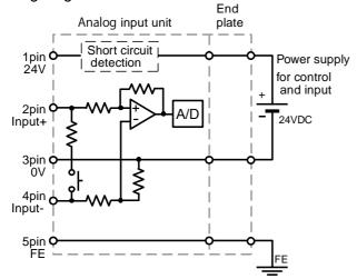
Input impedance Voltage input type: 100kΩ Current input type: 50Ω
