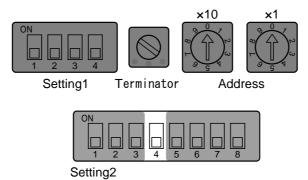
HOLD/CLR Switch : When a fieldbus communication error occurs or the communication idle state, all output can be set to Hold or Clear.
