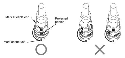
(3) Turn the connector clockwise. It stops when turned 1/4 turn.Turn it further. When the connector is turned 1/2 turn from the original position, the projected portion is set at the diagonal position to the mark and the turn is completed.
