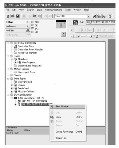
•[Select Module screen] is displayed. Select [ETHERNET MODULE Generic Ethernet Module], and click on [OK].
