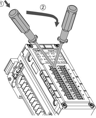
1 Insert a flat blade screwdriver inclined to the left into the right hole of the two holes as shown in the figure below.
