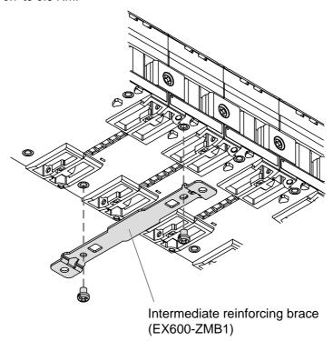
(2)Fix and tighten the end plates at one end of the unit. (M4)
