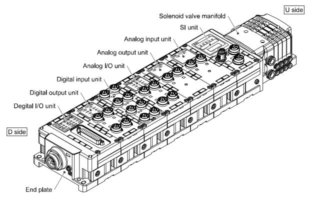
SI unit: Performs Fieldbus communication and solenoid valve manifold ON/OFF output.
