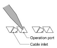
② Incline the screwdriver to the right as indicated by the arrow. When the screwdriver is pushed downwards until it stops, the cable inlet will open.
