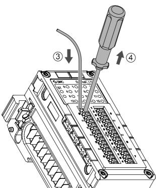
The electric wire below can be connected to the terminal block connector.
