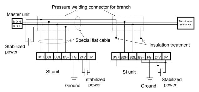
This SI unit is multi power supply type slave. It has 2 supplying sections for communication and solenoid valve. It's possible to supply power to the supplying section for communication by the special flat cable. But another power is needed at the supplying section for solenoid valve. Also, the power can be supplied from the supply power for solenoid valve to communication power supplying section.
