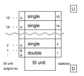
It is fixed depending on whether the solenoid valve carrying the manifold inside wiring is single or double.
