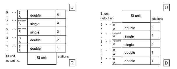
In the e.g. of wiring shown above, the 3<sup>rd</sup> ,4<sup>th</sup> single can be changed to double. In this case, the output no. of the 3<sup>rd</sup> solenoid valve on the B side will be 5, the output no. of 4<sup>th</sup> solenoid valve on the B side will be 7.
