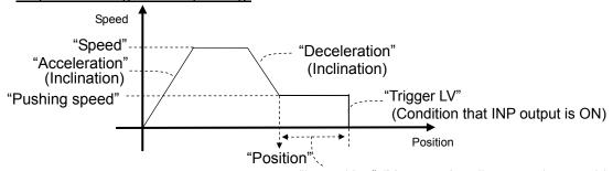
"In-position" (Max. moving distance when pushing)
