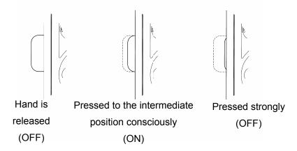
During the manual operation, if an unexpected actuator motion occurs, releasing or strongly pressing enable switch on the teaching box stops the actuator motion and the motor power turns off (servo OFF)
