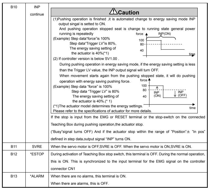
The table below shows the changes in the output signal with respect to controllers state.
