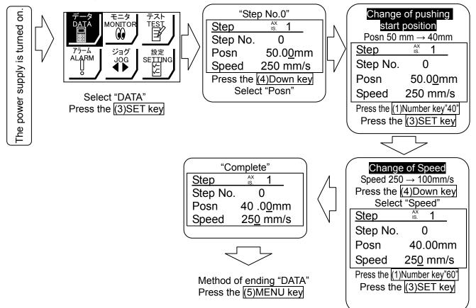
"Step No.1" / Positioning operation / At the time of shipment, Step No.1 is set to positioning operation
