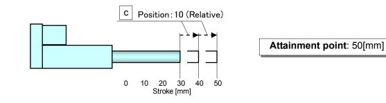
Condition 2) 30mm position  $\rightarrow$  **Step no.1**  $\rightarrow$  **Step no.1** (Move M: Relative)
