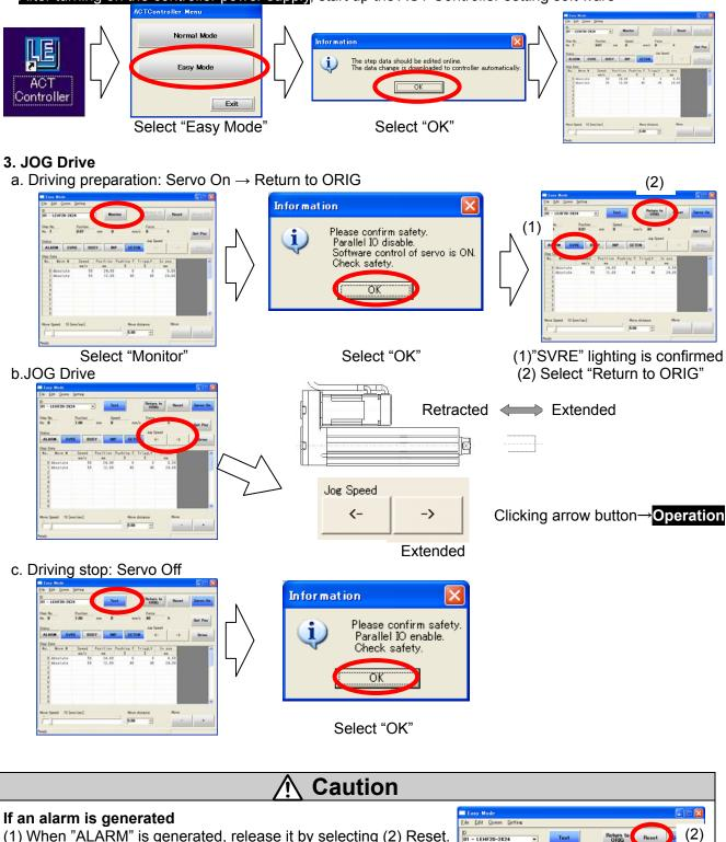
(1) When "ALARM" is generated, release it by selecting (2) Reset.
