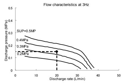
Recommended typical condition A: Calculate air pilot pressure in case of discharge rate 20L/min and pressure 0.15MPa
