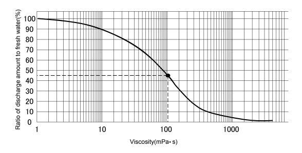
Recommended typical condition B: Calculate discharge amount of fluid with viscosity 100mPa•s in case of discharge rate 4.5L/min and discharge pressure 0.1MPa.
