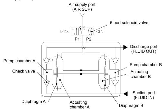
First, the air is supplied for switching valve mounted outside the pump. Then the signal is given from timer etc. and the air starts flowing into each actuating chamber in turn and moves diaphragm up and down.
