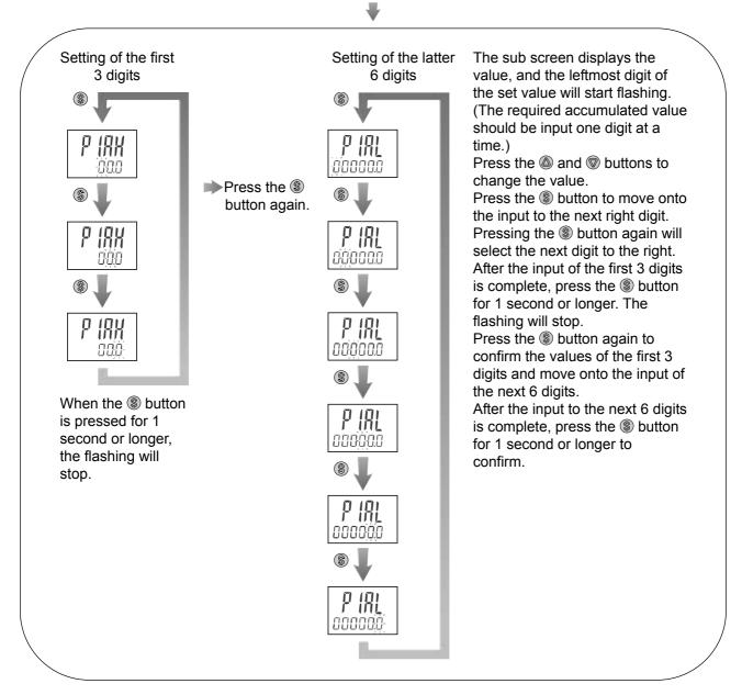
Press the S button to confirm.  $\P$  Move on to the selection of display colour.
