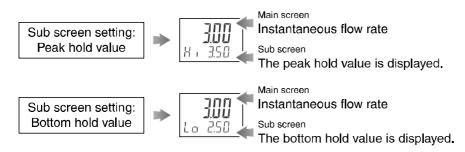
The maximum (peak) and minimum (bottom) flow from when the power is supplied to this moment is detected and updated.
