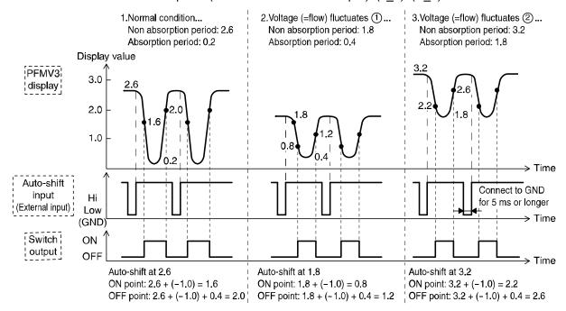
Setting range when auto-shift function is selected is -4.40 to 4.40. If relative set value after the auto-shift is out of upper or lower limit, this monitor operates with upper limit (5.10) or lower limit (0.70).
