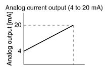
Min. rated flow Max. rated flow
