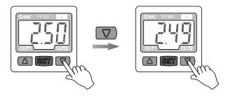
4. Press the button to finish the setting of OUT1. [n\_2] or [P\_2] is displayed to continue with settings for OUT2 as above.
