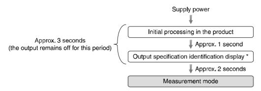
\*: Green: Flashes once. PF3W5□-□-1 (Analogue 1 to 5 V type: Without temperature sensor) Flashes twice. PF3W5□-□-2 (Analogue 4 to 20 mA type: Without temperature sensor) Flashes three times. PF3W5□-□-1T (Analogue 1 to 5 V type: With temperature sensor)
