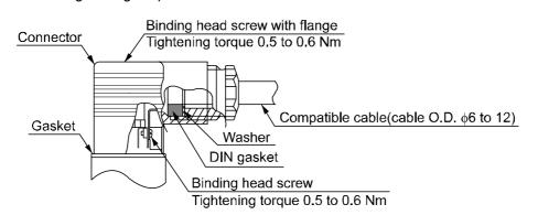
\*: Use after remove inner of DIN gasket in case of cable O.D. is )9 to 12.
