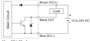
Max. 30V, 80mA Residual Voltage not exceeding 1V
