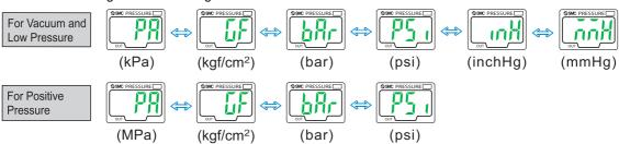
Press the SET button to set and to move on to setting a display color.
