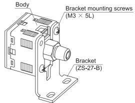
Mounting procedure with the panel mount adapter
