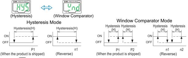
Press the SET button to move on to setting an output node.
