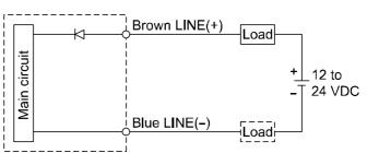
\*: Install the load either on the LINE(+) or LINE(-) side.
