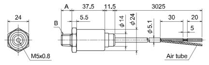
Be sure to release the air in the air tube of the cable to the atmosphere.
