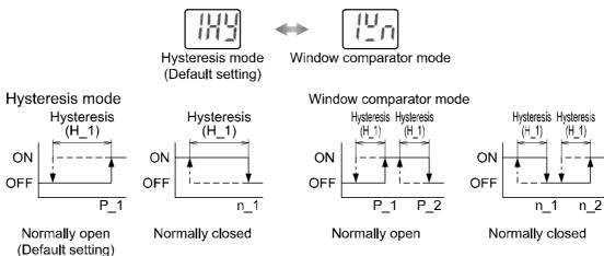
Press the SET button to set the selected operation mode, and the output style of OUT1 option will appear.
