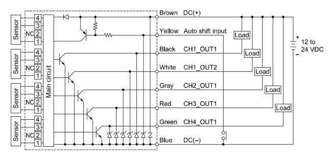
PSE201-(M)□: PNP open collector 5 outputs + Auto-shift 1 input Max. 80 mA
