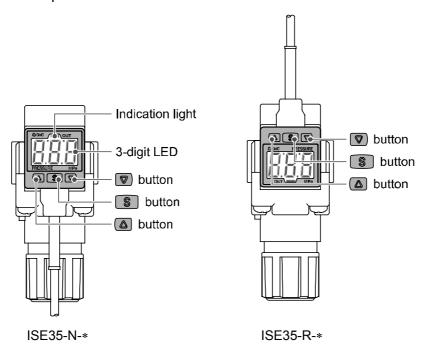
Indication light (Green LED): Displays the operation condition of the Pressure switch.
