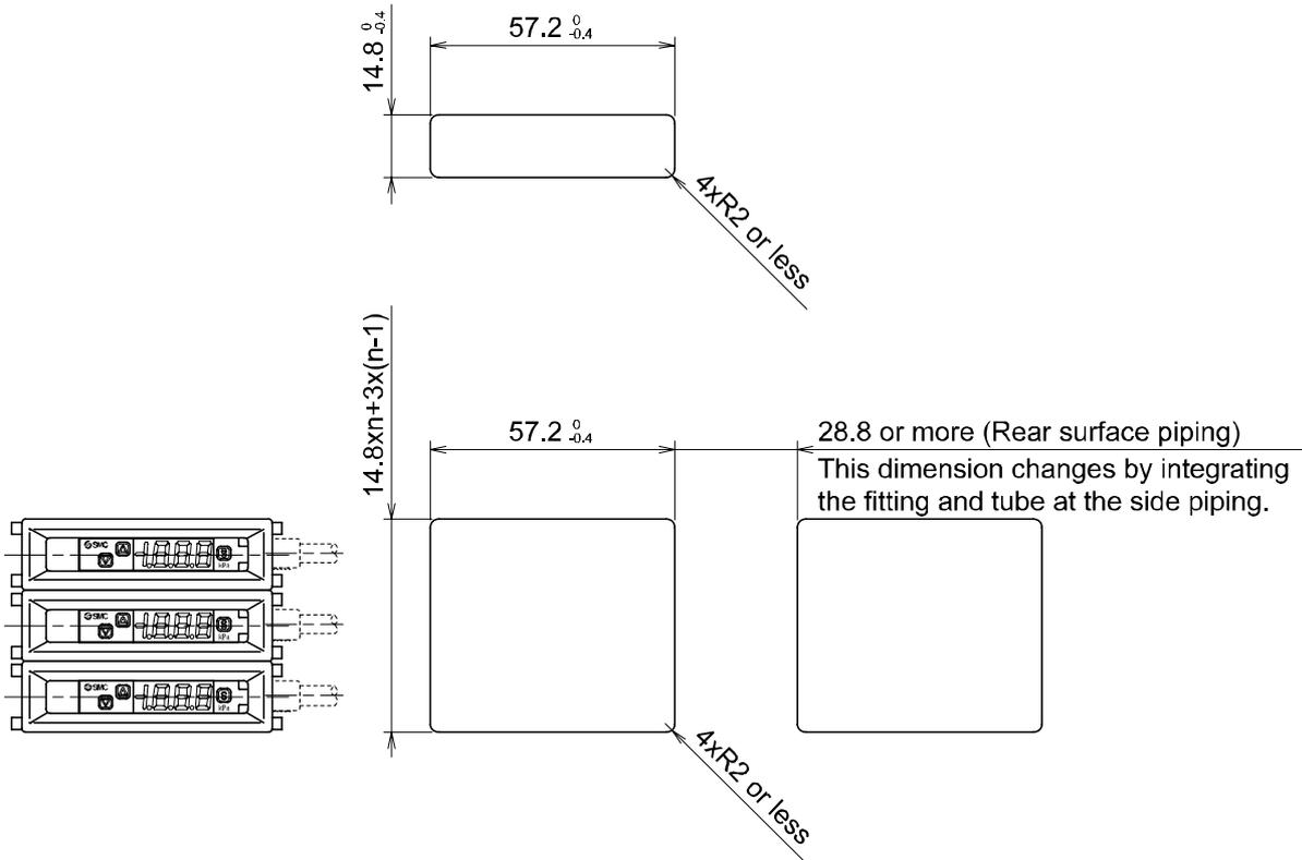
○DIN rail mounted side piping
