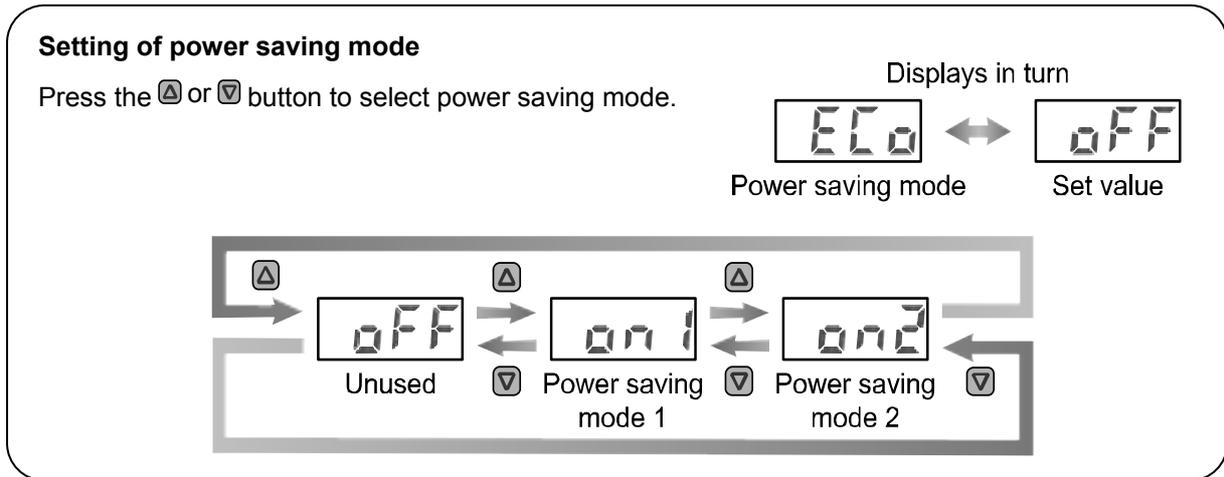
Press the  $\text{S}$  button to set.  $\Downarrow$  Return to function selection mode.
