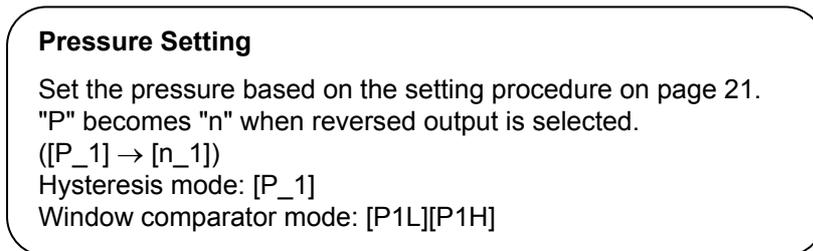
Press the  $\text{S}$  button to set.  $\downarrow$  Move on to setting of hysteresis.
