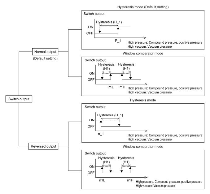
If the point where the switch output is changed is out of the set pressure range due to selection between normal and reversed output, hysteresis is automatically compensated.
