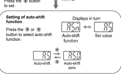
Press the § button to set. ¶ Move on to setting of effective output.
