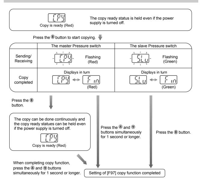
\*: If the copy to the slave Pressure switch is not completed, it is detected as a copying function sending/receiving error.
