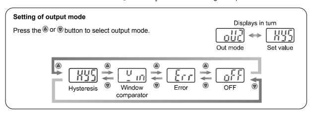
Press the § button to set. Move on to setting of reversed output.
