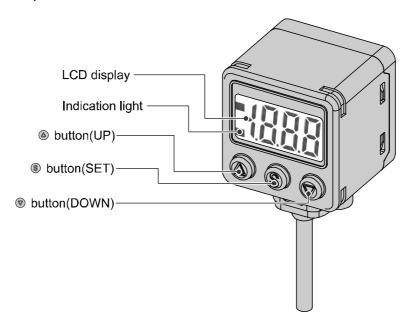
Indication light (Orange LED): Displays the switch operation condition.
