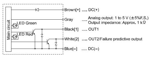
\*: The symbol shown in [] means the pin assignment of connector connection type.
