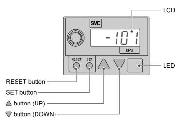
RESET button: Resets at error occurrence and for zero clear of the display.
