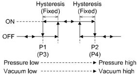
\*: •Hysteresis mode (same as for positive pressure use) When the value of hysteresis is set to 2 digits or less, the switching output might chatter due to fluctuation of the input pressure around its set point.
