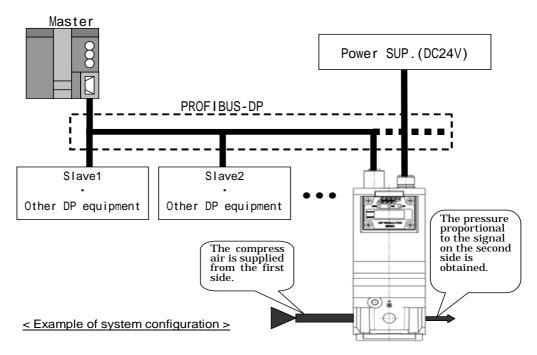
As shown in the structure example above, this product is to control air pressure for pneumatic equipment. Do not use it for any other application.
