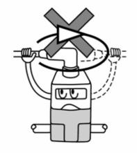
The right angle cable connector does not rotate. Do not rotate it.
