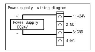
Select a DC power supply with adequate capacity with low ripple.
