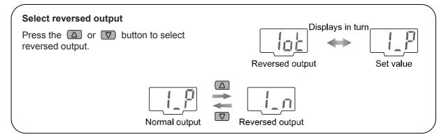
Press the **SET** button to set. **W** Moves on to charged potential setting.
