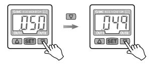
4. Press the **SET** button to finish the setting. Then [P\_2] is displayed. **Set** as above.
