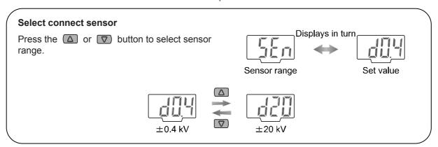
After selecting sensor range, press the △ and ▽ button together.
