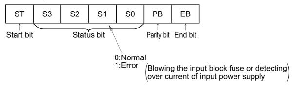
It is possible to confirm the peripheral fault error only by status register on the ADDR1 side for  $\mathsf{EX250}\text{-}\mathsf{SAS3}$  which occupy 2slaves.
