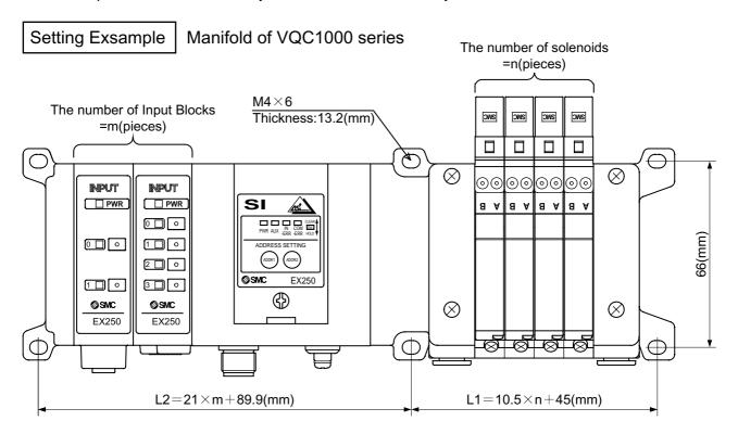
For example, the table below shows the size when manifold of VQC1000 series connected. Please refer to an individual catalog for the size when other manifolds are connected.
