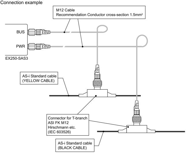
Neither M12 cable, As-I standard cable, nor connector for T-branch are supplied form SMC. Contact with each maker about the detail of the catalog etc.
